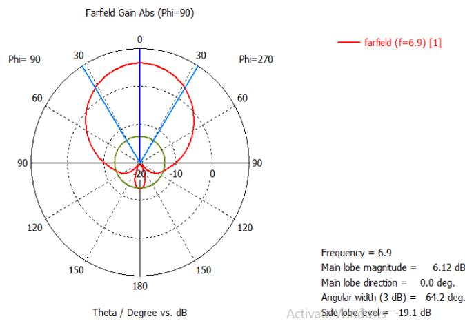
Fig 12: Polar plot of Gain at 6.9 GHz
