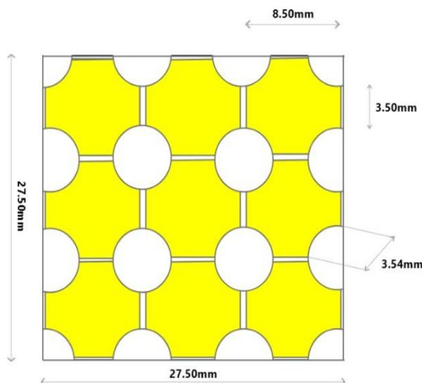
**Fig 2:** Layout of top substrate
