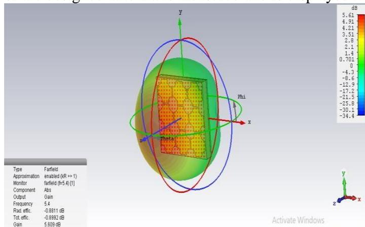
Fig 7: Gain at frequency 5.4 GHz
