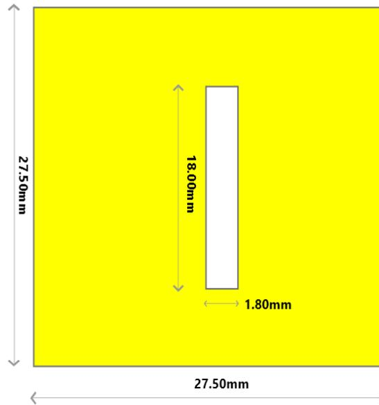
Fig 3: Layout of Ground plane
