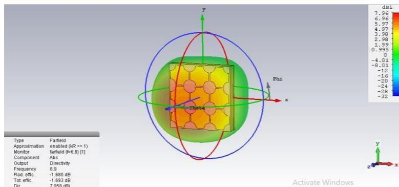
Fig 13: Directivity at frequency 6.9 GHz
