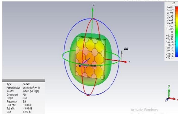
Fig 11: Gain at frequency 6.9 GHz
