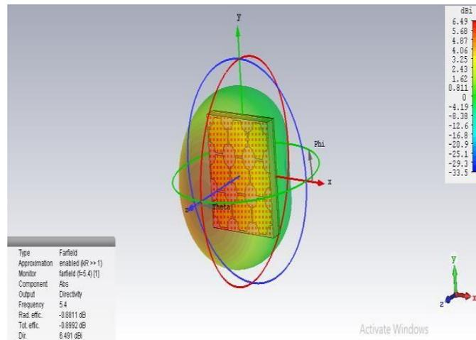
Fig 9: Directivity at frequency 5.4 GHz
