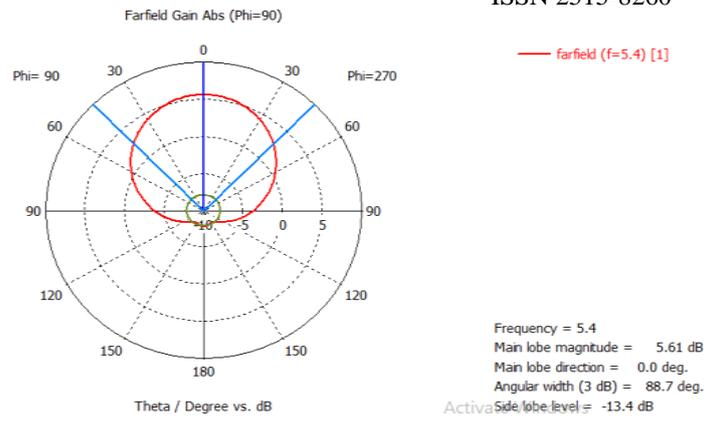
Fig 8: Polar plot of gain at 5.4GHz
