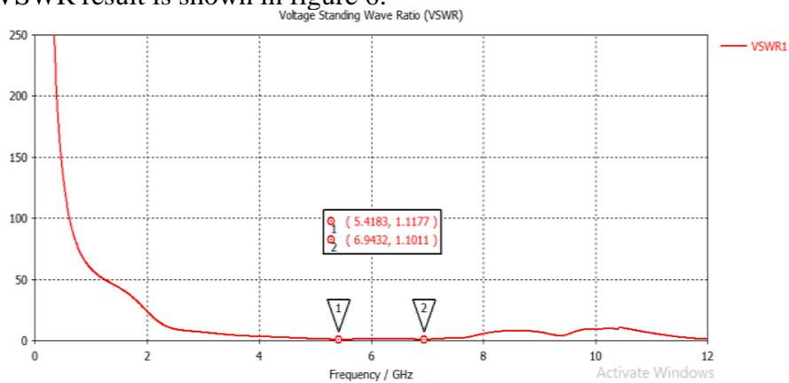
Fig 6: VSWR of EBG Patch antenna
