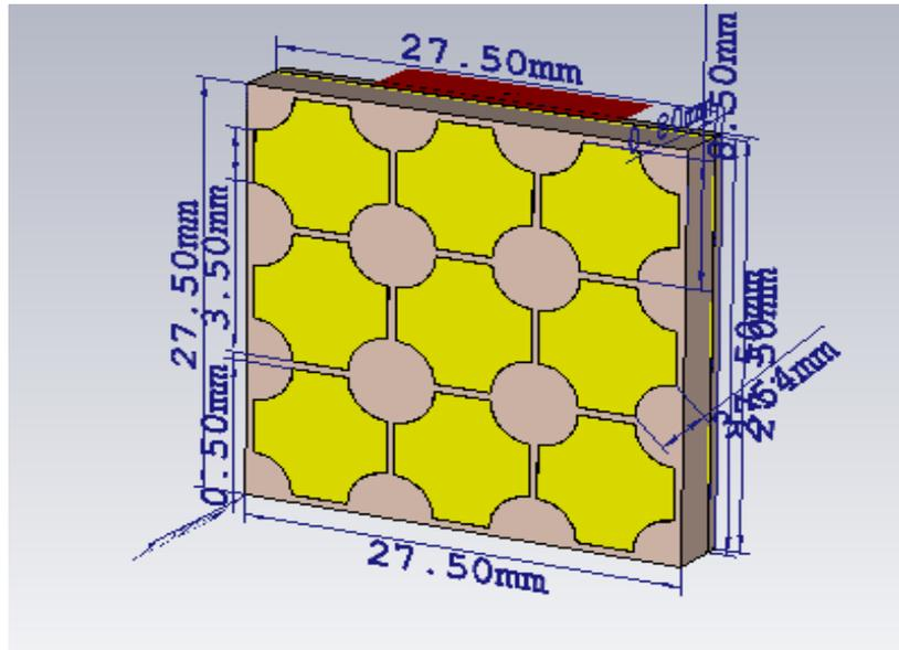
**Fig 1:** EBG aperture coupled antenna
