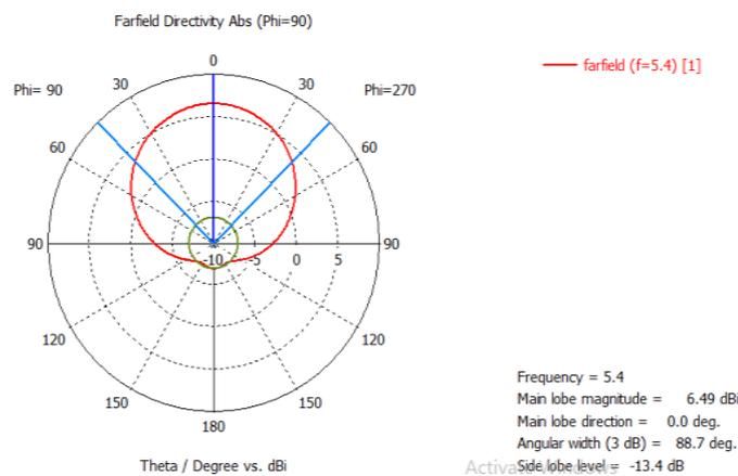
Fig 10: Polar plot of directivity at 5.4GHz
