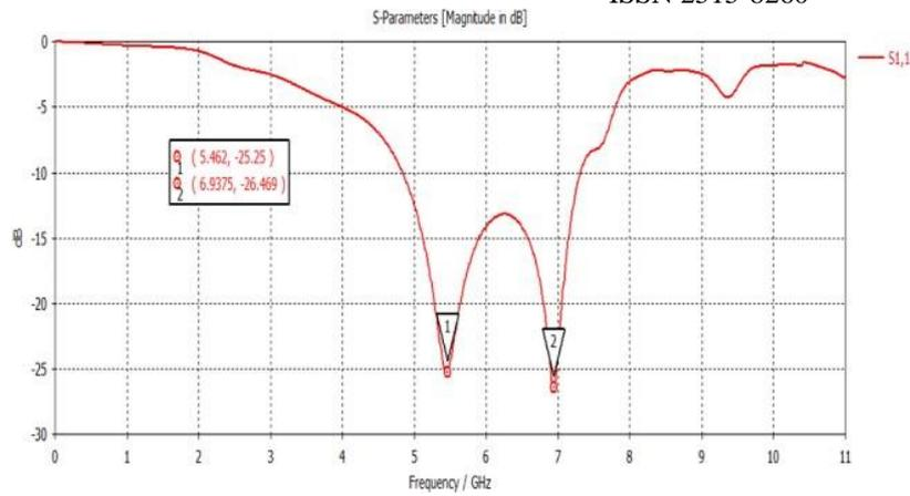
Fig 5: Return loss of EBG Patch antenna
