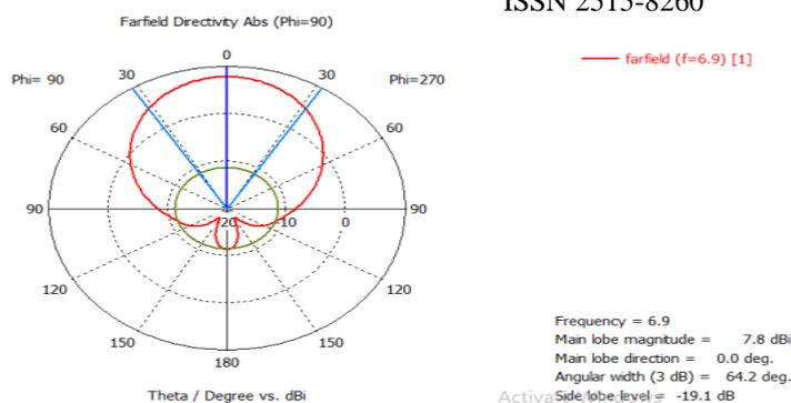
Fig 14: Polar plot of directivity at 6.9GHz
