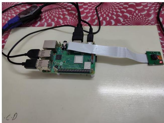
Fig 5 Kit and Pi camera connection
