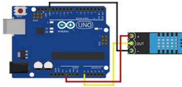
Fig 2 Arduino Uno with DTH-11
