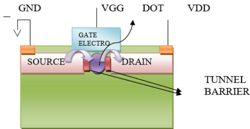
Fig.1 Structure of Silicon based SET
