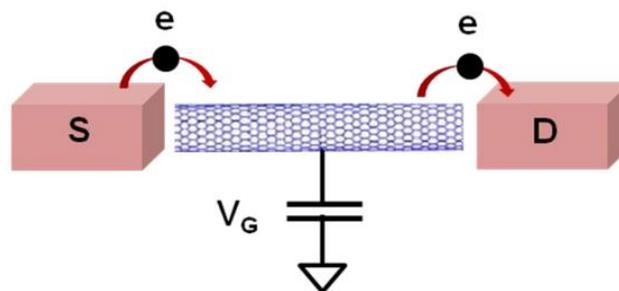
Fig.2 Structure of Carbon Nanotube SET
