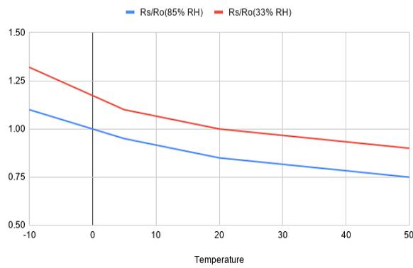
Fig 10.Rs/Ro Vs Temperature
