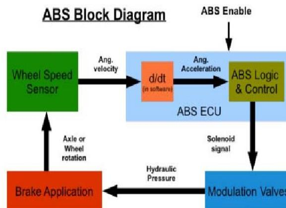
Fig 1. Antilock braking system
