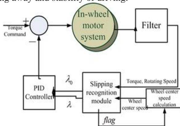
Fig 2. Acceleration skid control
