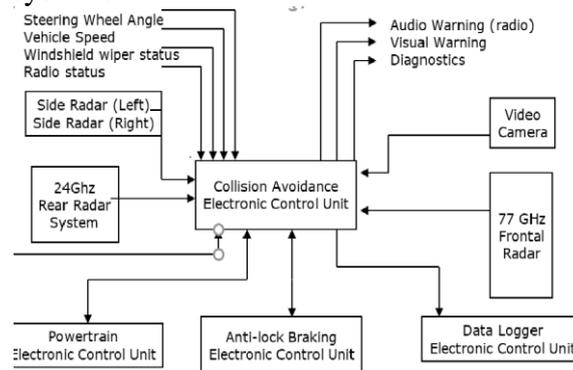
Fig 4. Forward collision warning system
