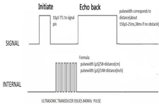
Fig 11.Ultrasonic sensor pulse diagram
