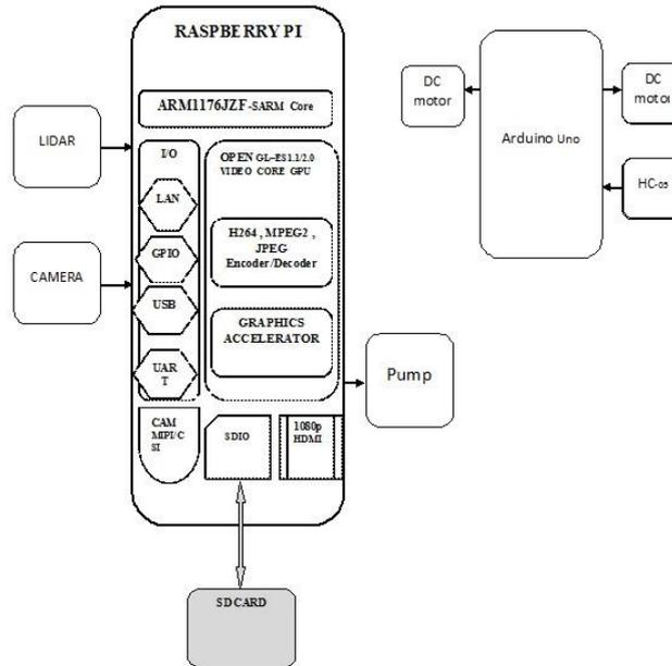
Fig. 1. Block diagram of the Robot
