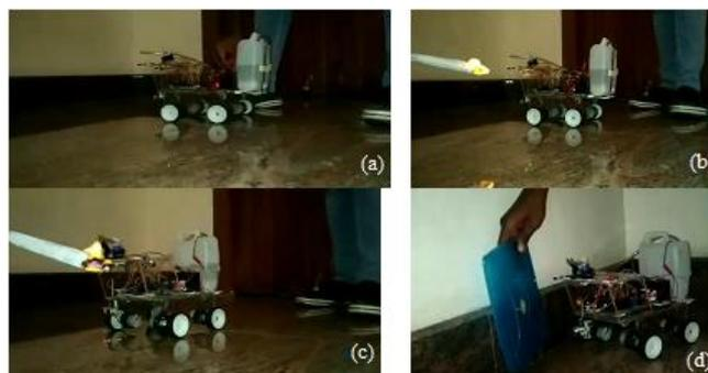
Fig. 4.a) Robot Reached the Destination, b)Robot sensing the Fire, c) Robot Fighting with Fir and d) Obstacle Detection
