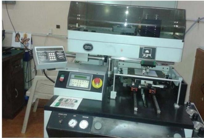
Fig.3 Sensor strip making machine
