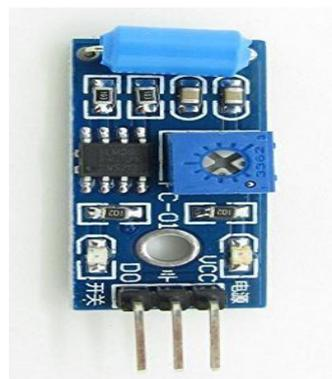
Fig 6: Vibration Sensor
