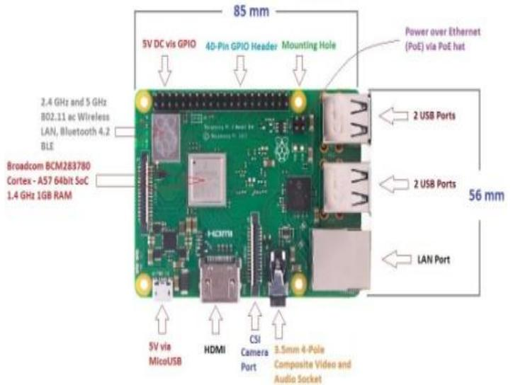
Fig 3: Pin Out Diagram Rpi
