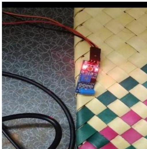
Fig 11: Vibration Sensor
