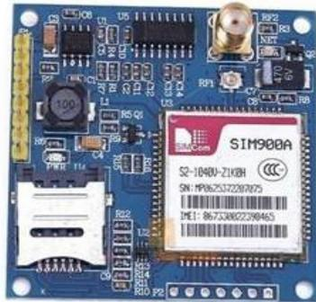
Fig 5: GSM Module
