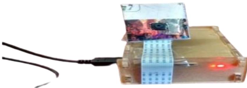
*Fig 4 prototype alarms when driver feels dozy*
