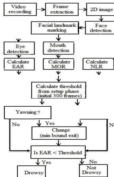
**Fig 1** The block diagram of the drowsiness detection system
