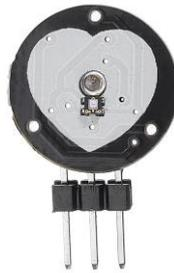
Fig 3.2 Pulse sensor
