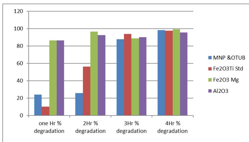
**Fig. 5:** 200ppm o-cresol removal using mixed MNP
