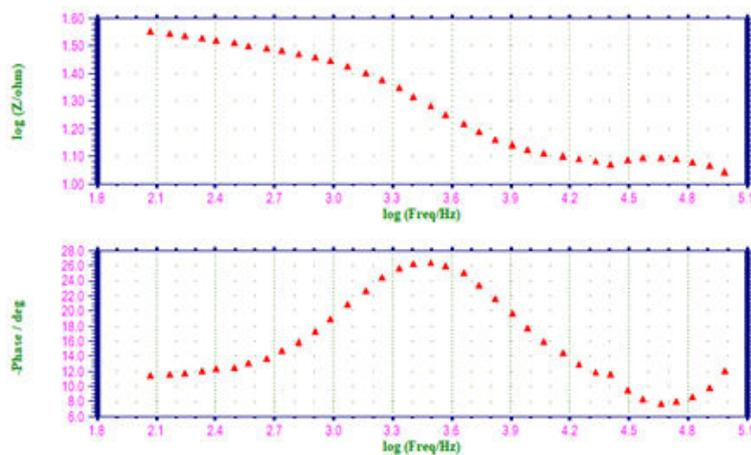
**Figure. 3a: AC impedance spectra of mild steel immersed in sodium chloride solution (Bode Plot).**
