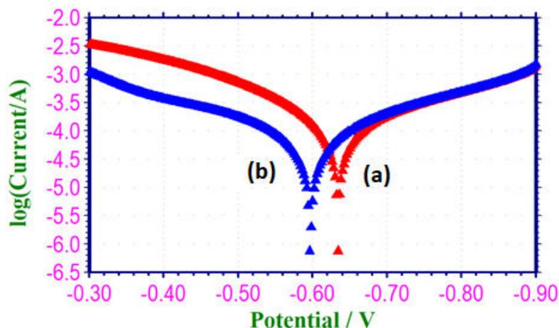
**Figure. 1: Potentiodynamic polarization curves for corrosion of mild steel in sodium chloride solution in absence and presence of AEPL inhibitor (a) Mild steel in sodium chloride solution (blank) (b) Mild steel in sodium chloride with 10% aqueous extract of AEPL**
