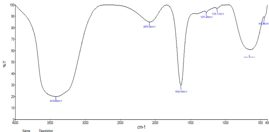
**Figure. 4b: FTIR spectrum of scratched film from the mild steel surface after immersion in sodium chloride solution with 10% aqueous extract of AEPL**
