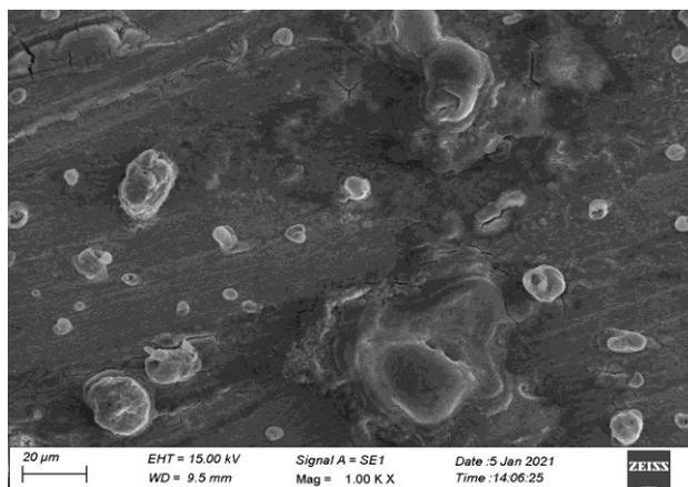
**Figure 5b: SEM image of mild steel specimen after immersion in sodium chloride solution (blank)**
