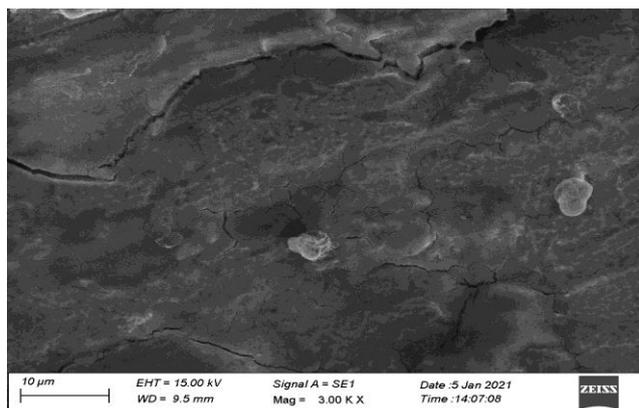
**Figure. 5c: SEM image of mild steel specimen after immersion in sodium chloride in the presence of 10% aqueous extract of DMPL.**
