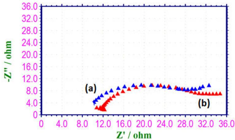
**Figure. 2: AC impedance spectra of mild steel immersed in sodium chloride solution in the absence and presence of AEPLE inhibitor (Nyquist plots)(a) Mild steel in sodium chloride solution without inhibitor (b) Mild steel in sodium chloride solution with 10% aqueous extract of AEP leaves.**
