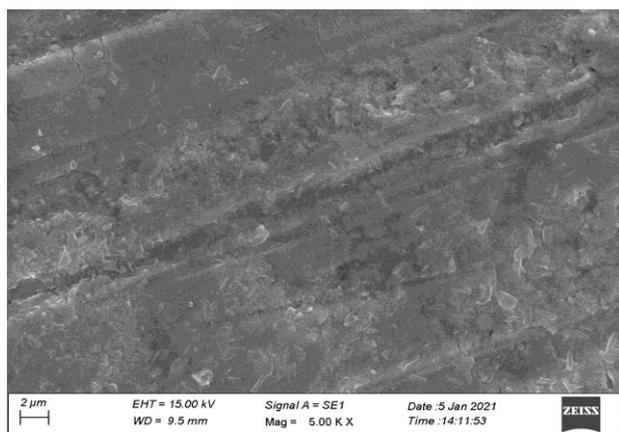
**Figure. 5a: SEM image of polished mild steel specimen before immersion in sodium chloride (control)**
