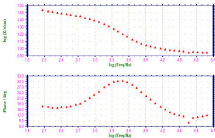
**Figure. 3b: AC impedance spectra of mild steel immersed in sodium chloride solution with 10% aqueous extract of AEP leaves (Bode Plot)**
