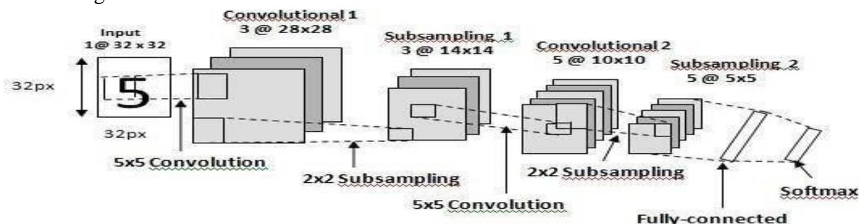
Figure1. Architecture of CNN
