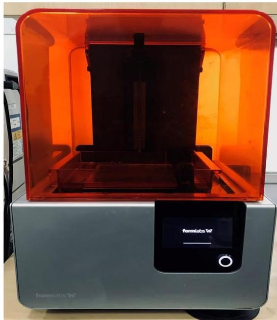
**Figure 1: SLA 3D PRINTER (FORM2 FORMLAB)**
