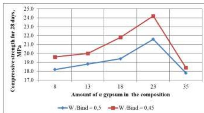
Figure 1. Dependency of the strength of CGB brick on the amount of alpha gypsum
