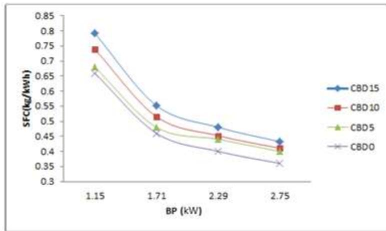
Figure.3. BP in KW vs Specific fuel consumption in kg/kWh
