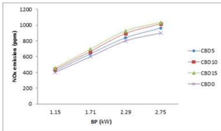
Figure.6 BP in kW vs NO<sub>x</sub> emission in ppm
