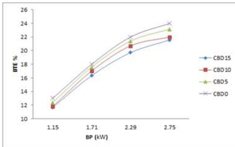
Figure.2. BP in kW vs BTE in %
