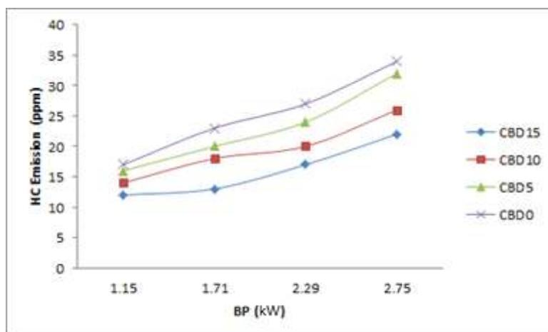
Figure.7 BP in kWvs HC emission in ppm
