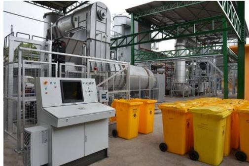
**Figure 3** Combustible Incinerator Plant in the Clinwaste facility (Image courtesy of Clinwaste (M) Sdn. Bhd.)
