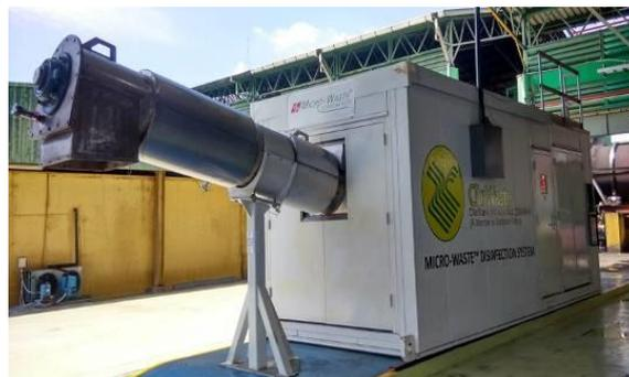
**Figure 4** The AMB Ecosteryl 250 model in the Microwave Treatment Section in the Clinwaste facilities (Image courtesy of Clinwaste (M) Sdn. Bhd.)
