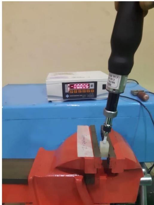
Figure 3. Testing the specimens using digital torque wrench
