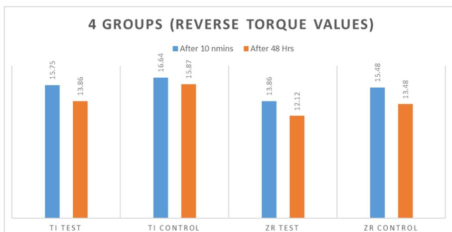
Figure 4. Mean reverse torque values of test and control groups
