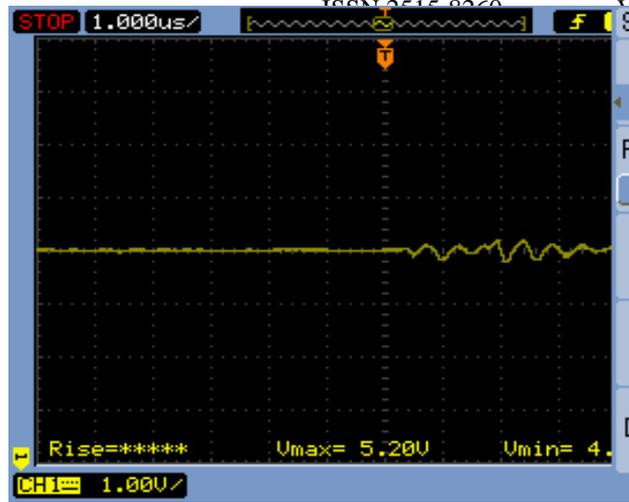
Figure. 2: Noise in LDR Sensor when bent.
