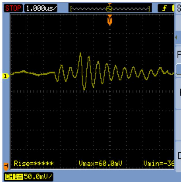
Figure. 3: Noise in Passive IR Sensor when bent
