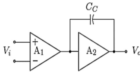
**Figure 5.** Block diagram of two-stage op-amp
