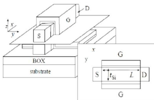
**Figure 3.** Fin-FET structure with a perspective over the entire fin
