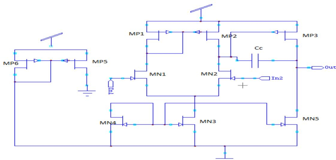
**Figure 7.** Proposed architecture of two-stage FinFET op-amp schematic circuit along with compensation circuit technique
