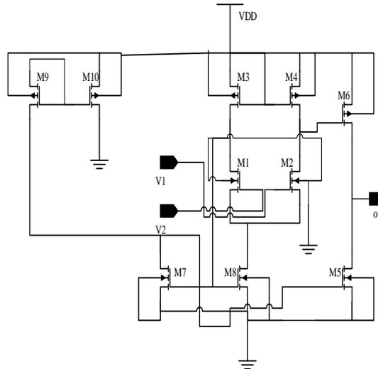
**Figure 6.** FinFET op-amp proposed for two-stage offset circuit
