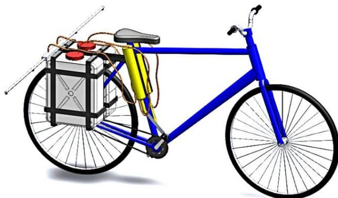
Figure 1. Design of bicycle powered sprayer
