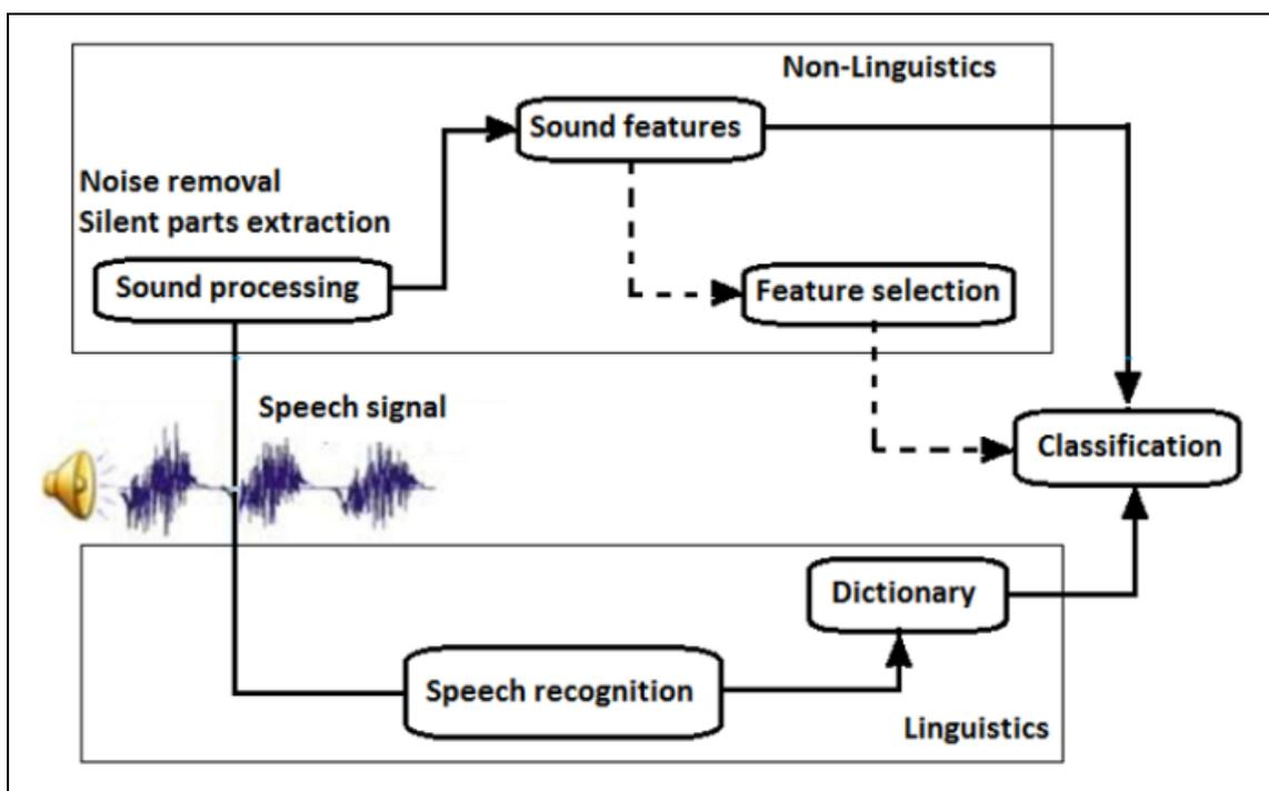
Figure 1 Architecture Diagram
