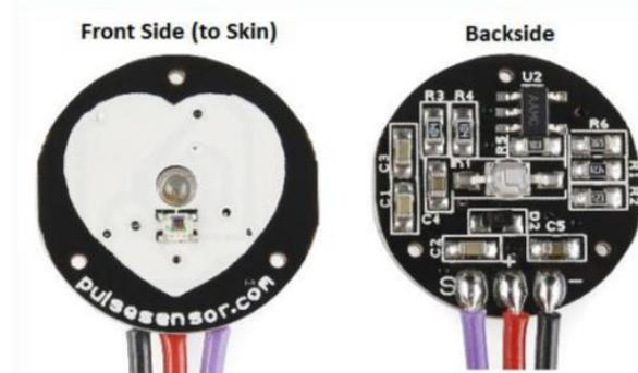
Fig. 4. Pulse rate sensor.
