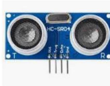
Fig. 8. Ultrasonic Sensor
