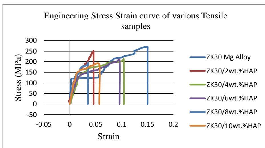
Fig.1 Engineering Stress strain curves of various tensile samples
