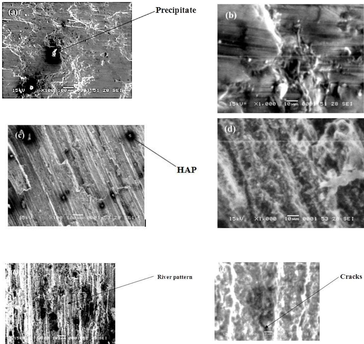
Fig.4 SEM Images of Compressive Fracture Surfaces of (a, b) ZK30 Mg Alloy, (c, d) ZK30/2wt%HAP, (e, f) ZK30/8wt%HAP
