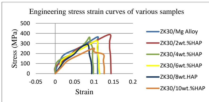
Fig.3 Engineering Stress Strain curves of various compressive samples
