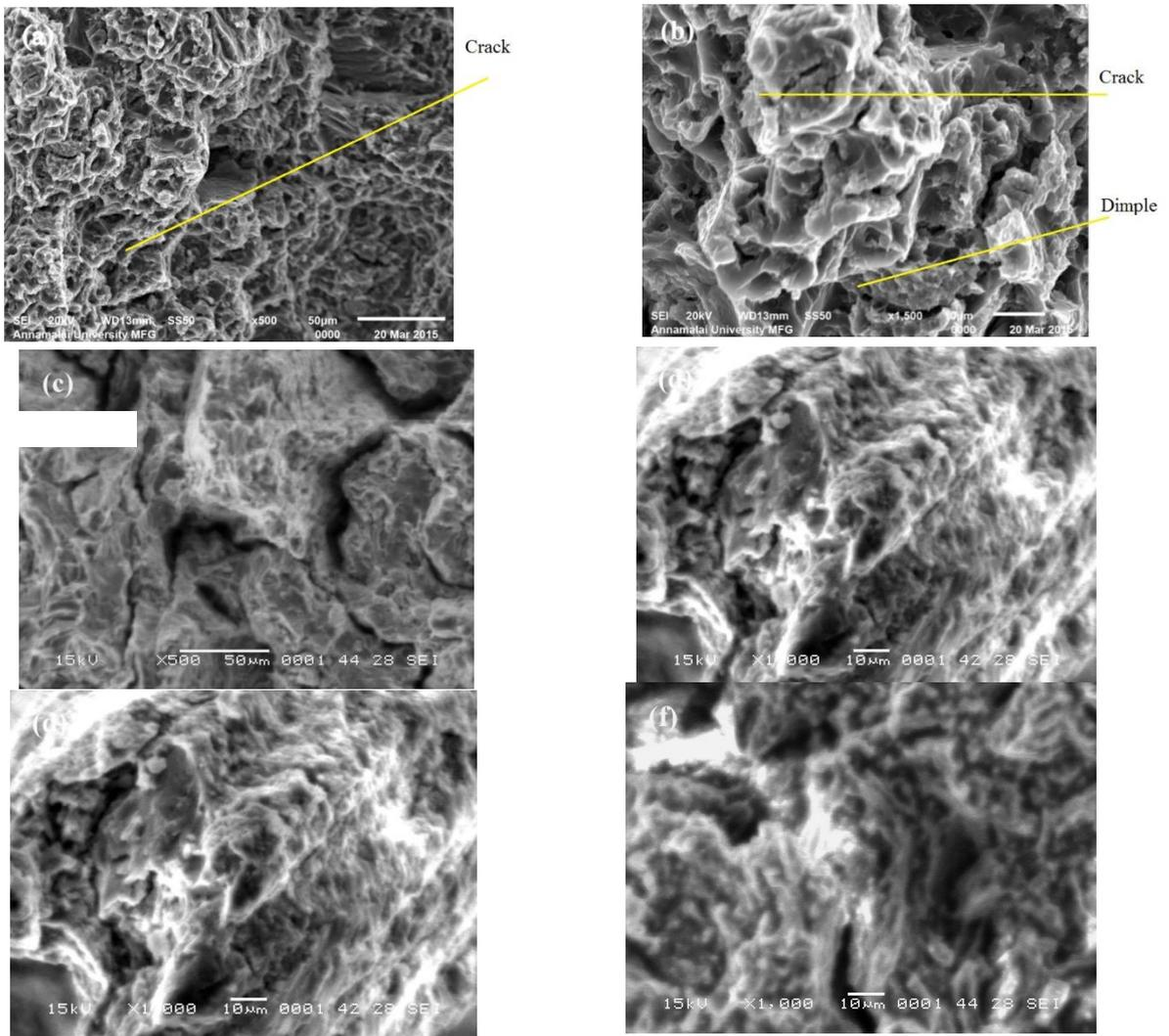
Fig.2 SEM Images of Tensile Fracture Surfaces of (a, b) ZK30 Mg Alloy, (c, d) ZK30/2wt%HAP, (e, f) ZK30/8wt%HAP
