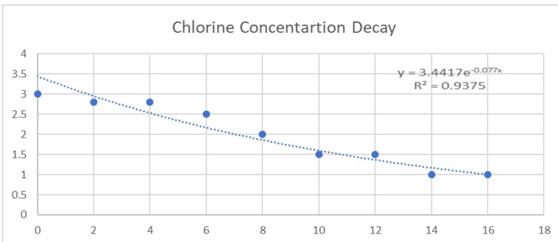
**Figure 2. Variation of Chlorine Concentration Decay with Time**
