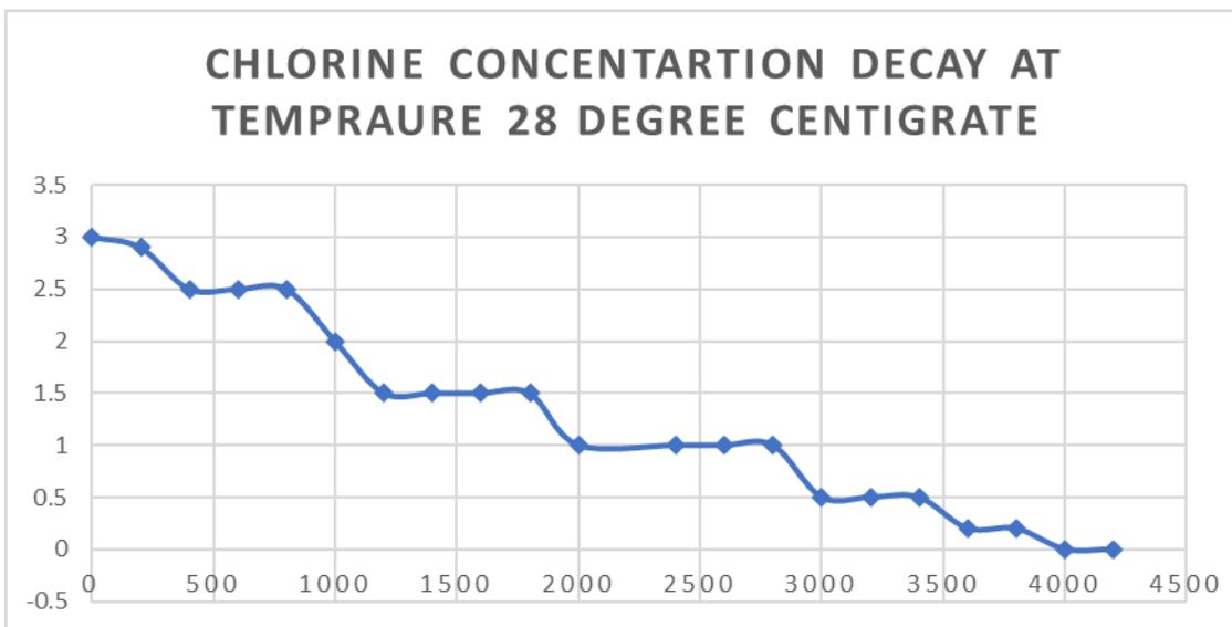
**Figure 1: Variation Chlorine Concentration Decay at Different Time Intervals.**
