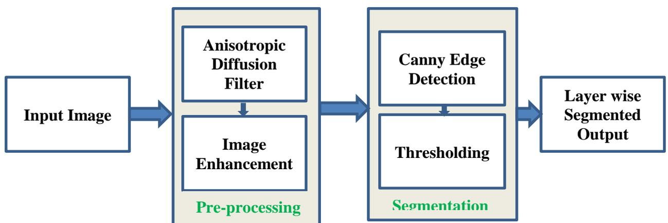
Figure 1: Block Diagram of the Experimental Method
