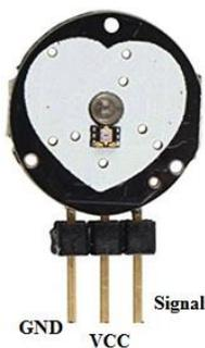
Fig.9. Pulse sensor
