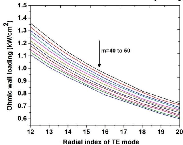
FIGURE 1. Ohmic wall loading for high order TE modes (RF power= 1000 kW, cavity length= 13 mm, λ= 1.25 mm).
