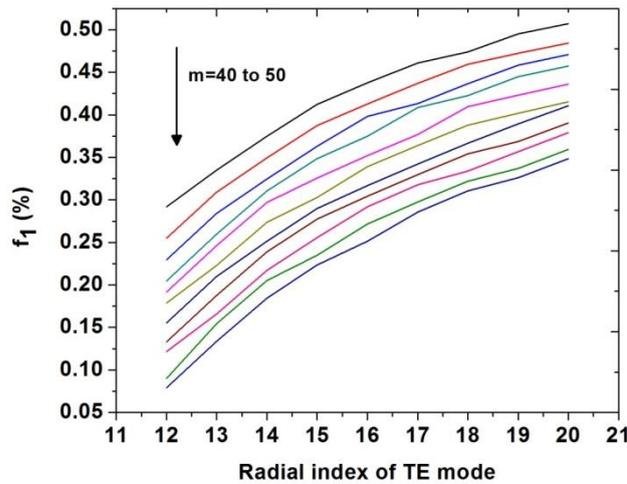
FIGURE 3. Frequency separation for high order TE modes.
