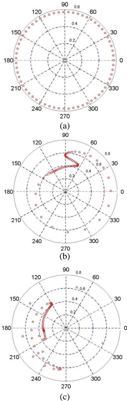
FIGURE7:The azimuthal phase bunching of electrons at different positions of the cavity.
