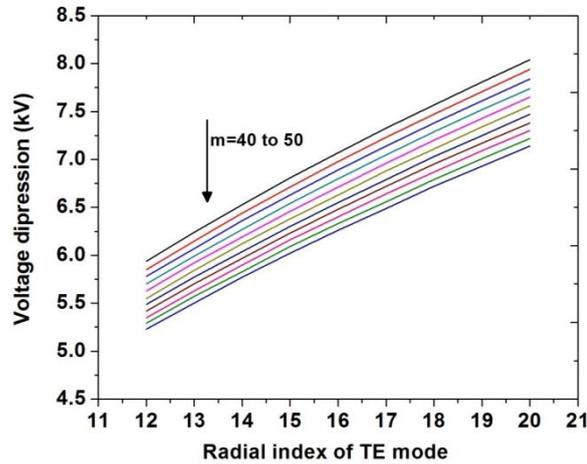
FIGURE 2. Voltage depression for high order TE modes ( $I_b= 40$  A,  $V_b= 90$  kV,  $R_c= 22.66$  mm,  $R_b= 9.53$  mm).
