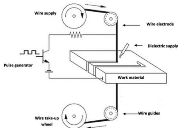
Figure 1 Working Principle Wire cut EDM Process [11]
