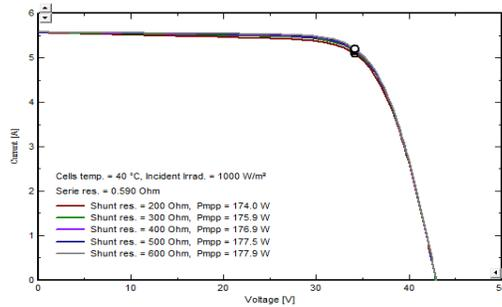
**Fig. 9. Current –Voltage characteristics for various shunt resistance**
