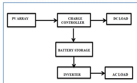
**Fig. 1. PV array with battery storage powering DC and AC loads**
