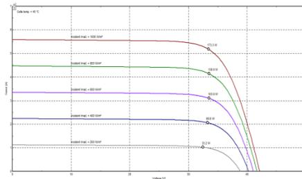
**Fig. 2. Current –Voltage characteristics**
