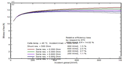
Fig 12. Efficiency –Incident global characteristics for various series resistance
