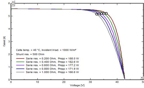
**Fig. 8. Current –Voltage characteristics for various series resistance**
