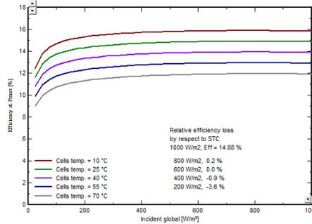
**Fig 7. Efficiency –Incident global characteristics for various cells temperature**
