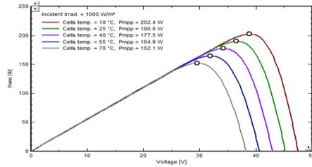
**Fig.6 power – voltage characteristics for various temperatures**
