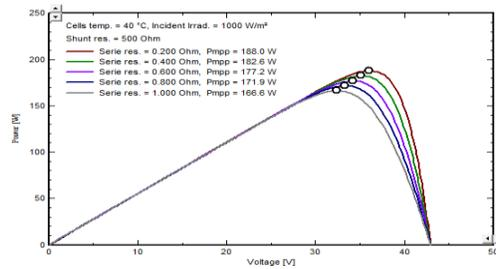
**Fig 10. Power - Voltage characteristics for various series resistance**
