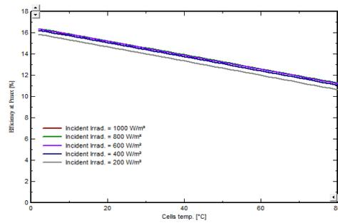
**Fig 4. Cells temperature – Efficiency at P<sub>max</sub> characteristics for various incident irradiance**
