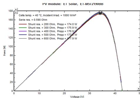
**Fig 11. Power - Voltage characteristics for various shunt resistance**
