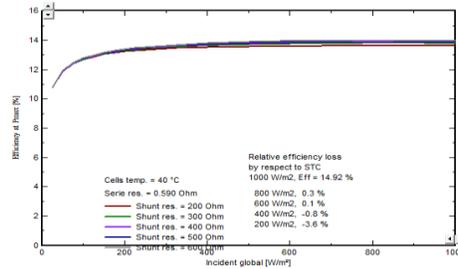
Fig 13. Efficiency –Incident global Characteristics for various shunt resistance
