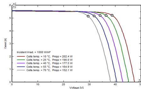
**Fig.5. Current –Voltage characteristics for various temperatures**
