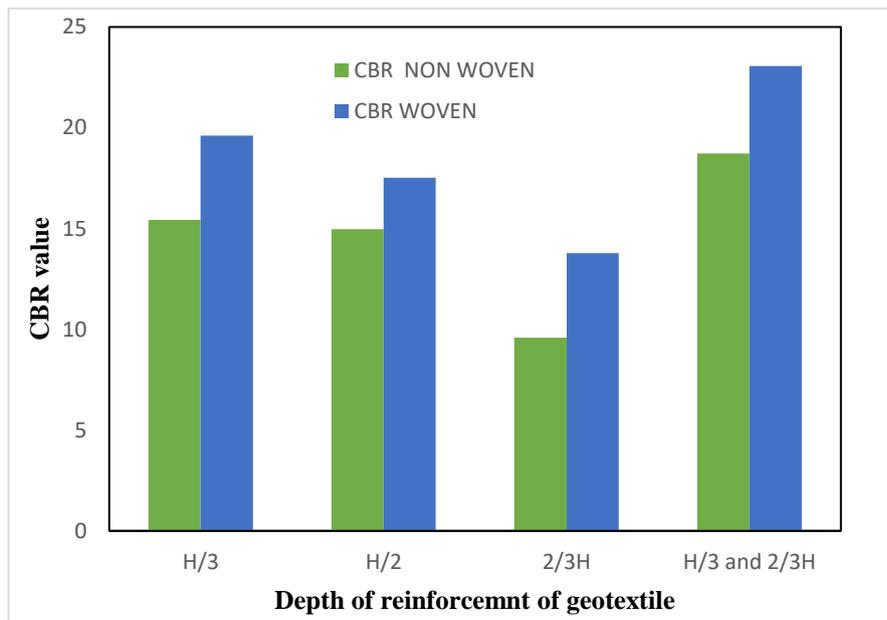
Figure 2 Plot of CBR values vs position of reinforcement
