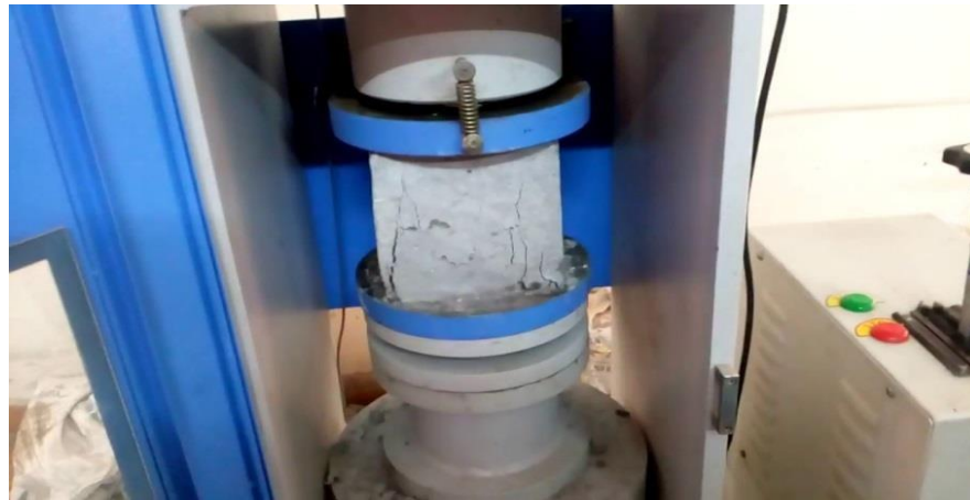
Figure 2. Compressive Strength Test
