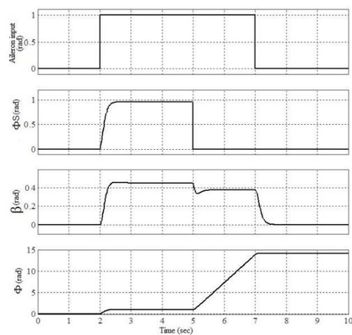
**Figure4.** FCS states with sensor fault (without reconfiguration)
