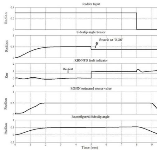
**Figure8.** Sideslip angle sensor fault at 5s at 0.36 value (for 747 Jet transport aircraft model)
