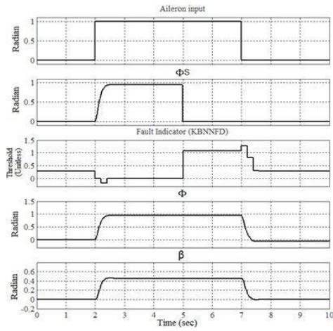
**Figure5.**  $\phi$  sensor stuck fault at 5s at '0' value
