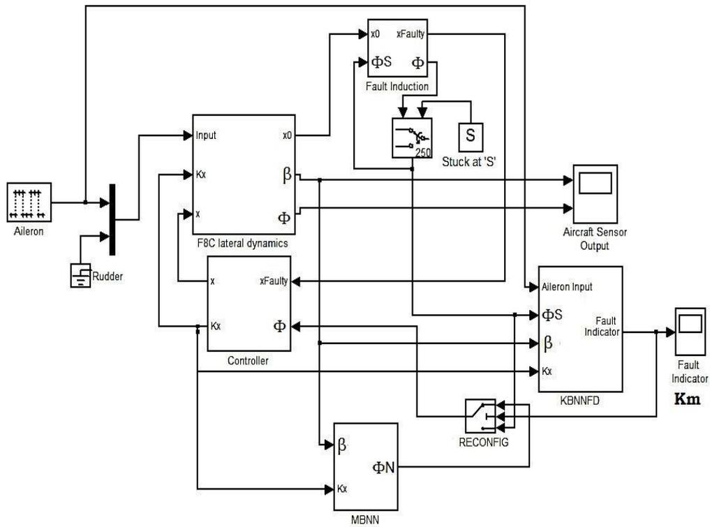
**Figure 2.** F8-C Lateral dynamic's Simulink model of NNSFA
