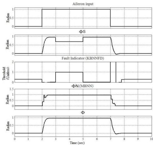
**Figure7.**  $\phi$  sensor intermittent stuck fault from 3 to 5s at '0.7' value
