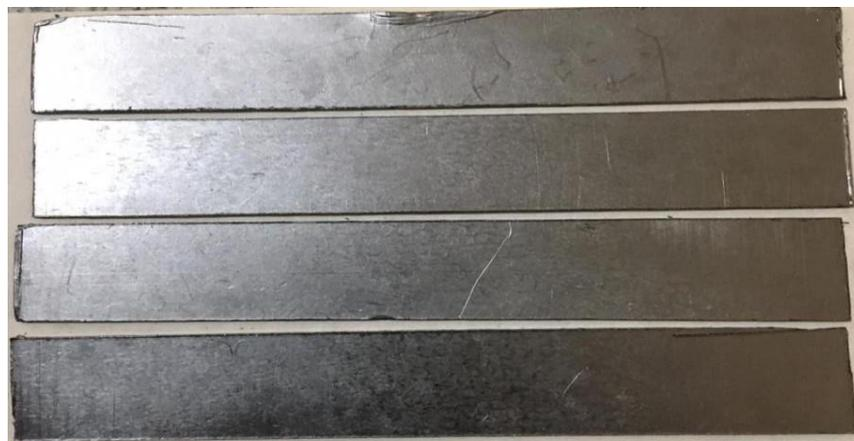
**Figure 1. Graphite Plate Electrodes**
