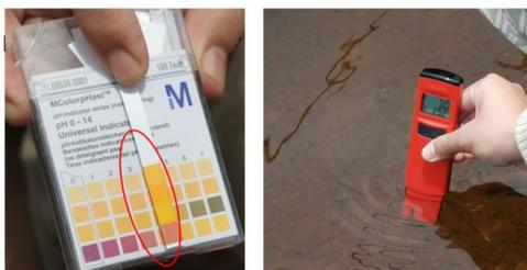
Fig. 1 1pH Measurement of Water Sample
