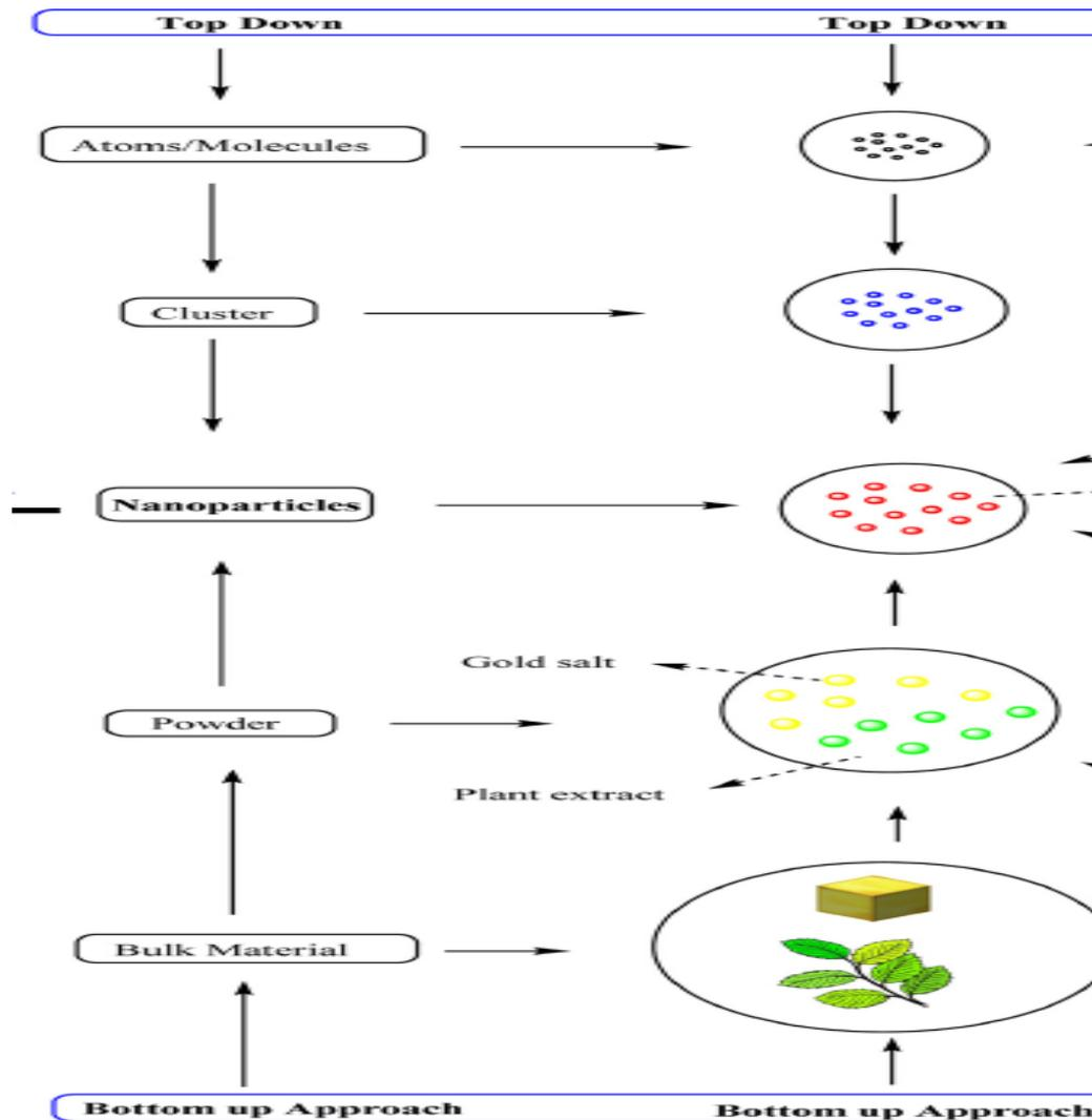
Fig. no. 6: Manufacturing of the gold nanoparticles by different methods (Dan Song, 2019)
