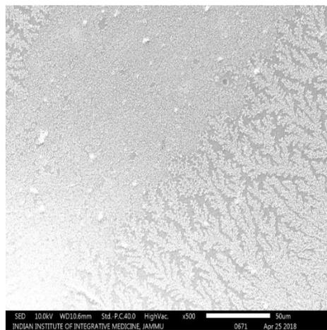
**Figure:** SEM of single-layered chitosan-nisin coated LDPE
