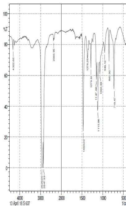
**Fig:** FTIR of single coated LDPE
