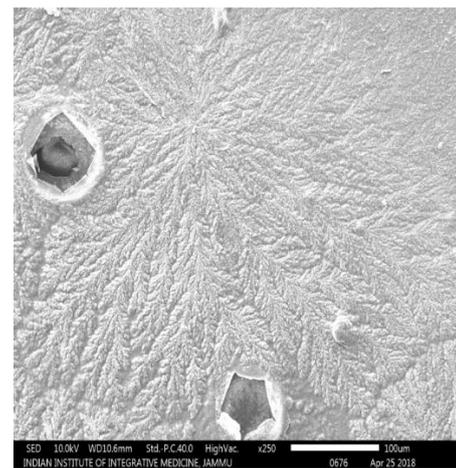
**Figure:** SEM of triple-layered chitosan-nisin coated LDPE
