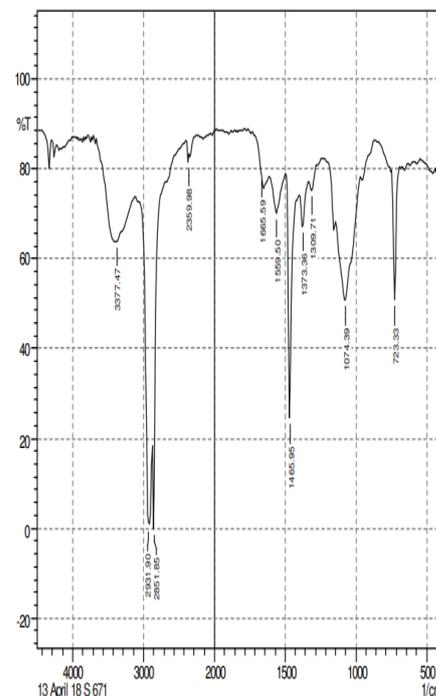
**Fig:** FTIR of triple coated LDPE
