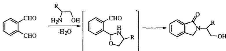
The reaction was done between alpha- amino alcohols and 2-formylbenzoic acid. To proceed the reaction equimolar amounts of the mixture of two components were heated at reflux in toluene solvent to obtained desired product.
