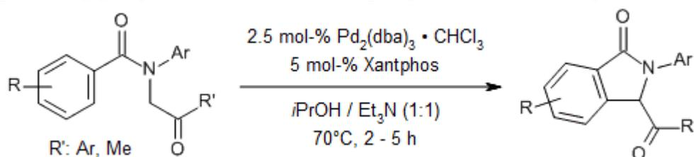
3-acyl isoindolin-1-ones and 3-hydroxy-3-acylisoindolin-1-ones can be produced with the help of an efficient reaction that is catalysed by palladium and there is cyclization within the molecules of 2-iodobenzamides with an addition of 2-oxoethyl function group on the atom of nitrogen under mild conditions in good yield.<sup>16</sup>
