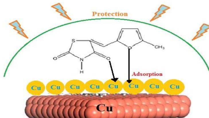
Fig.3. Adsorption of thiazole derivative 5-(5'-methylfurfurylidene-2')-2,4-dioxotetrahydro-1,3-thiazole on Cu surface
