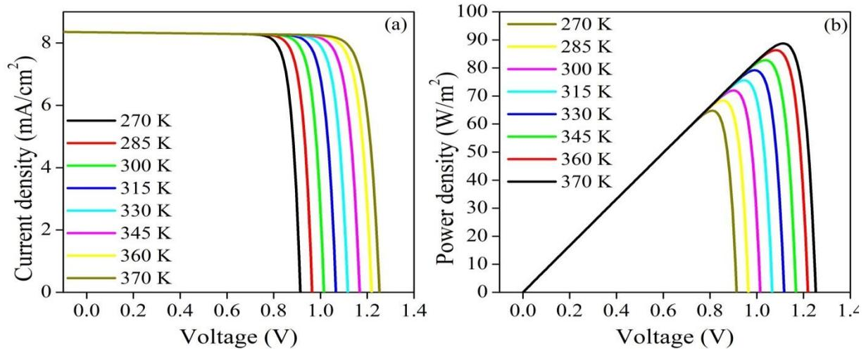
**Figure 1 (a) IV and (b) PV characteristic curves of PSC at different temperatures (from 270 to 370 K)**
