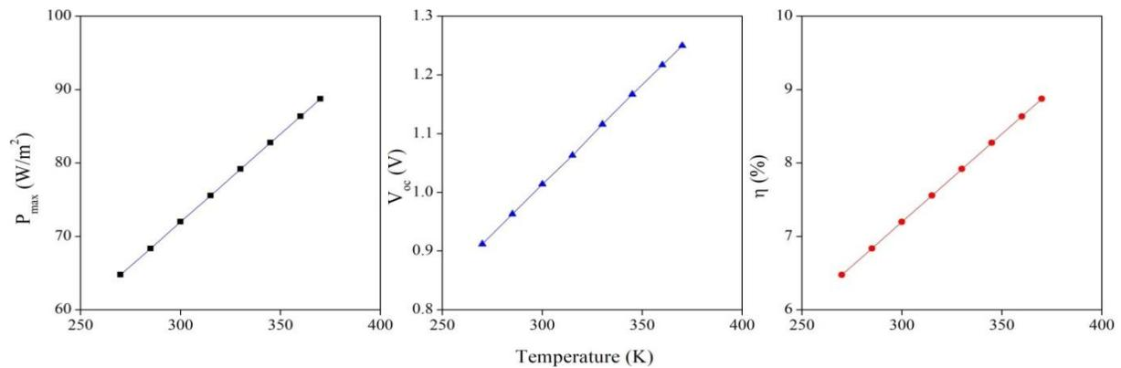
**Figure-2: Variation of (a) maximum power, (b) open circuit voltage and (c) efficiency of perovskite solar cell operated between the temperatures 270 and 370 K.**
