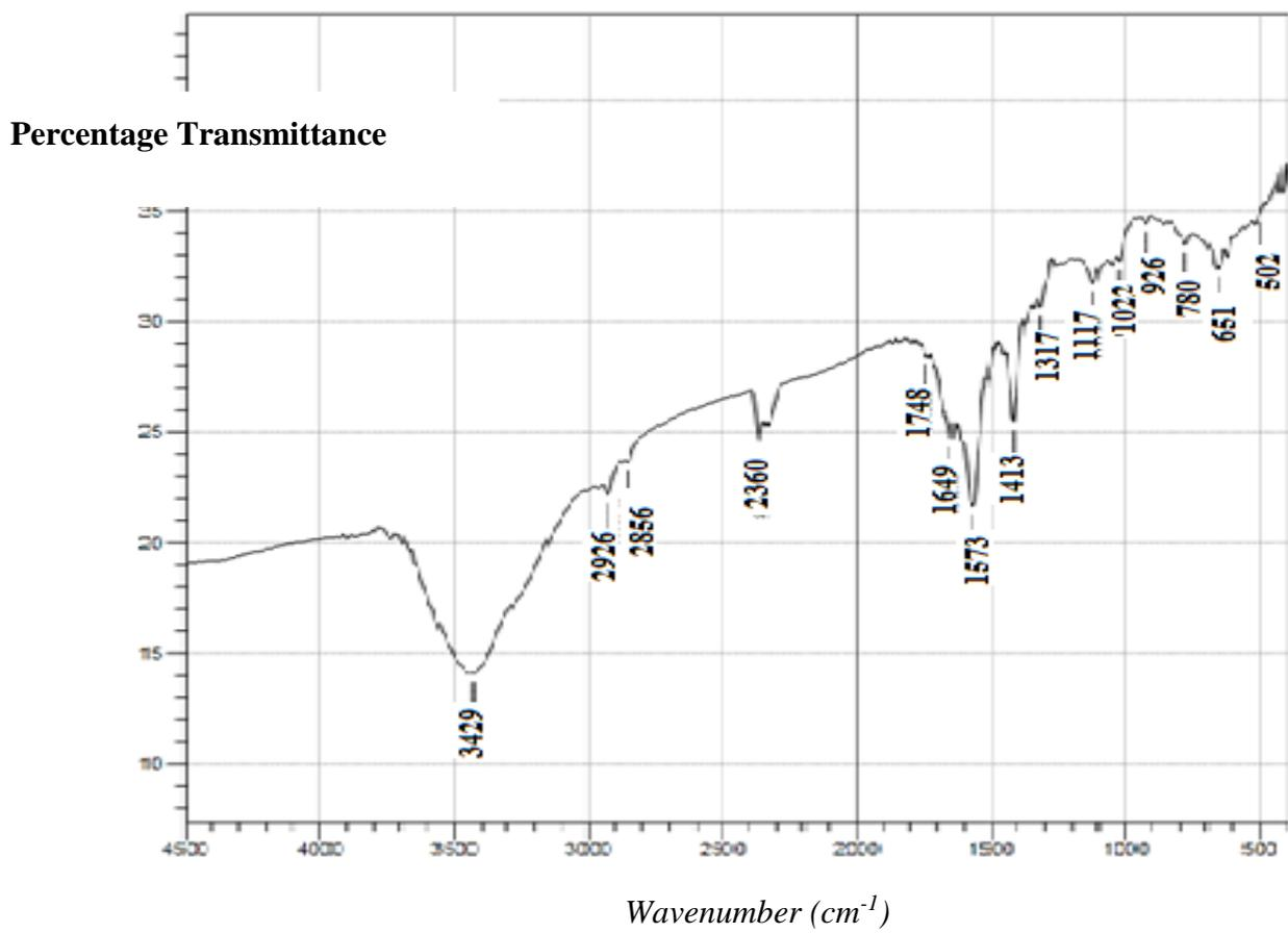
Fig 2: FTIR Spectra of Nylon 66
