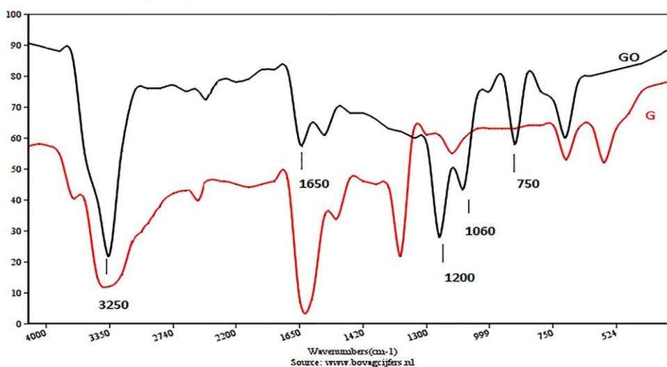
Figure 1- The FT-IR spectrum [1] graphite (G) and [2] graphene oxide I (GO)
