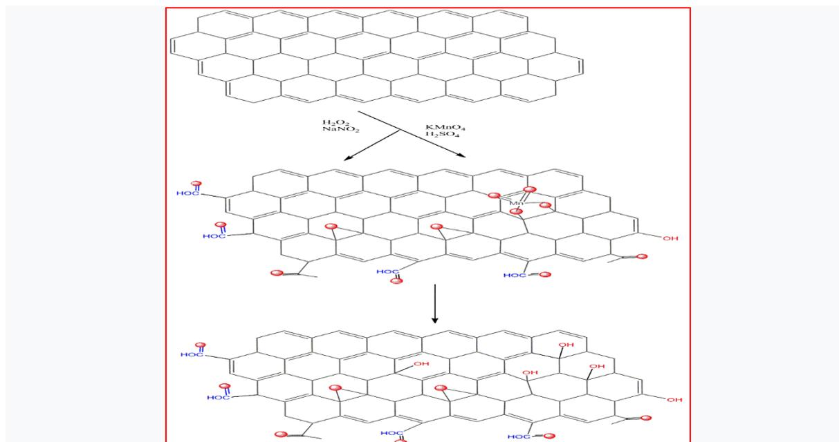
**Scheme 1-** synthesis of graphene oxide (GO) Nanoparticle (I) by Hummer's method from graphite
