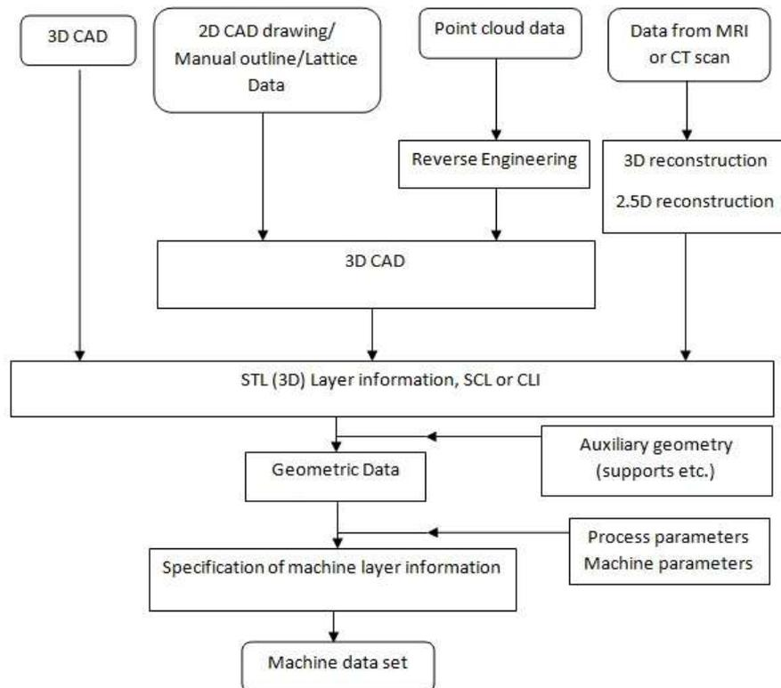
Figure 1 Additive Manufacturing Process flow chart
