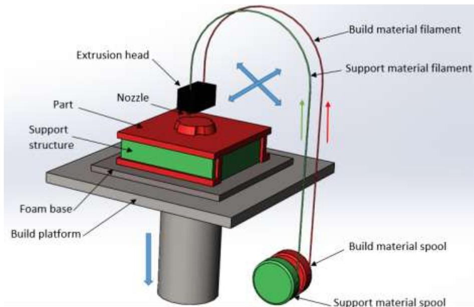
type of FDM machine used. This preprocessing is done for every layer of the model individually. For each layer, the FDM software generates the "tool path" for the movement of head. The preprocessed file generated by the FDM software (STL file) is sent to the FDM machine for part building.
