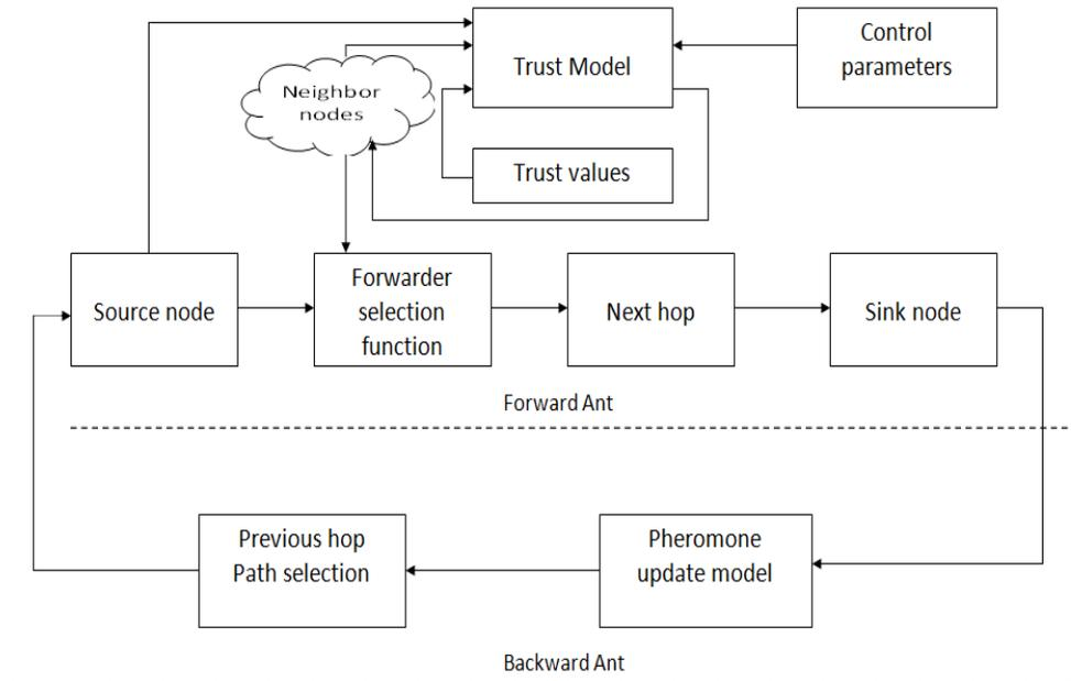
Figure 1: ACO based efficient routing framework.
