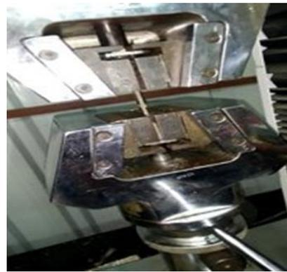
Fig-4(b): Micro tensile testing machine
