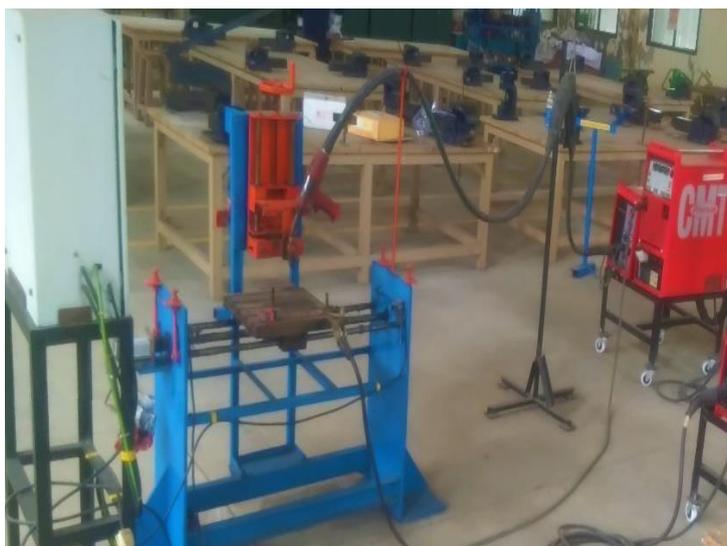
Fig-1: Cold Metal Transfer Apparatus setup
