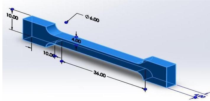
Figure-3: Tensile test specimen with ASTM standards
