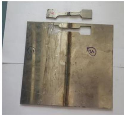
Fig-4(a): Tensile test specimen and welded specimen
