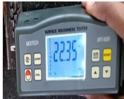
Fig-5(b): Roughness tester
