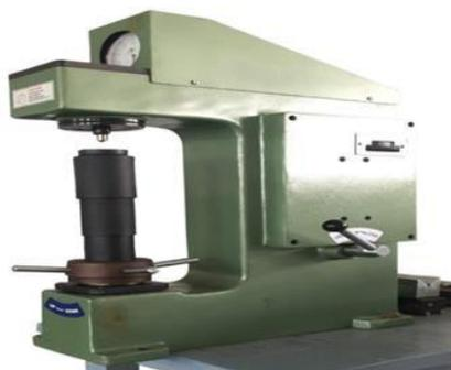
Fig-5(a): Hardness testing Machine
