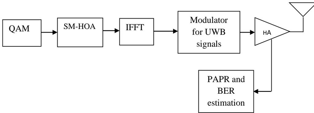
Fig 5. Proposed MB-OFDM-UWB hybrid system.
