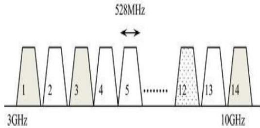
Fig:2 Multiband in UWB
