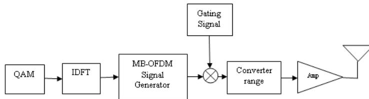
Fig 3. Transmitting side of MB-OFDM UWB signal [3].
