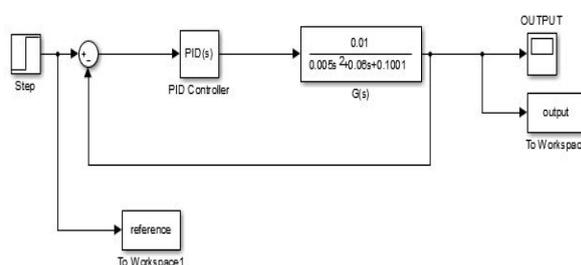
Fig 6. The graphical programming model of Chemical Reaction Optimization PID Algorithm
