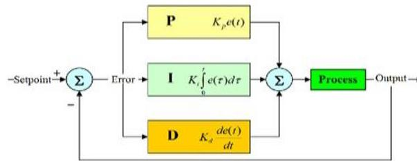
Fig2. PID Controller Block Diagram
