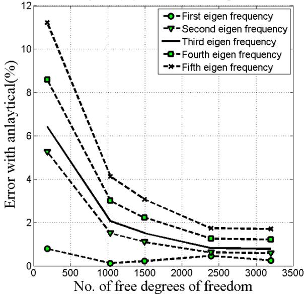
Figure 3. Convergence analysis of cracked circular domain discretized with 3-edge triangular and 4-edge quadrilateral elements.
