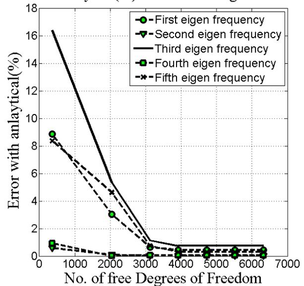
Figure 4. Convergence analysis of circular domain discretized with 8-edge triangular and 12-edge quadrilateral elements
