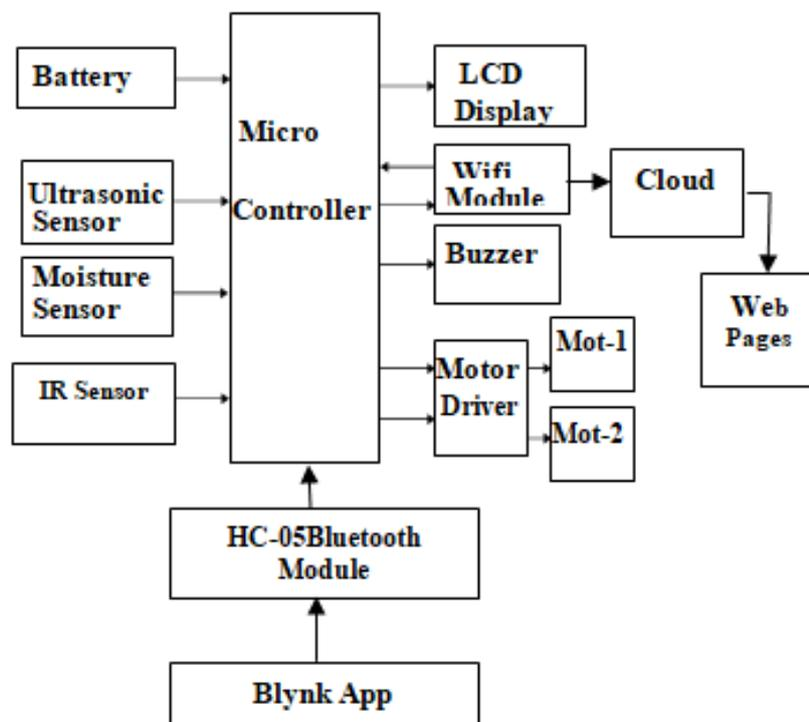
Figure 1: Block diagram of Garbage Collection and Monitoring Robot Using Wireless Communication
